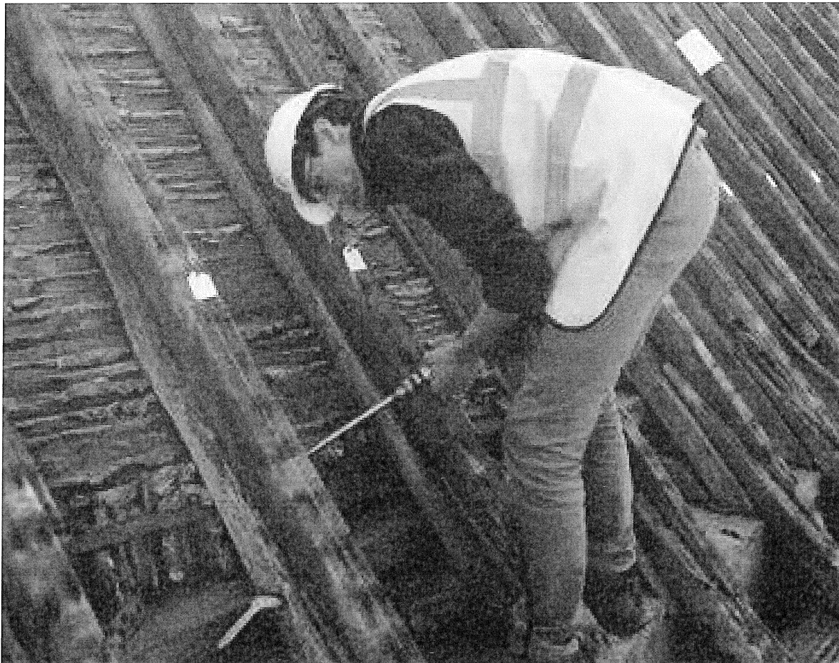
Ross Cook of the Oxford Dendrochronology Laboratory sampling roof timbers at The Vyne; this roof is over the Oak Gallery. © National Trust/Gary Marshall
